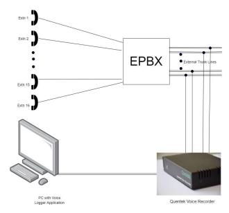
When connected at the Extension side, the recorder is capable of monitoring and recording extension side lines.
