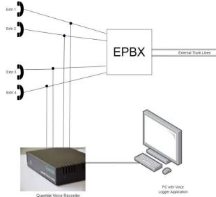
In both these modes, Quentek Voice Recorder is capable of logging call details including the Caller ID, Trunk Name, Ring Duration, Call Duration, Call Start Time & End Time, Call Type (Incoming/Outgoing) & Call Status (Failed/Missed/Connected),
